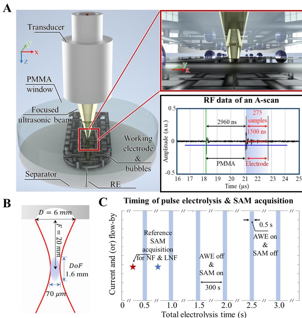
**Figure 3. The schematic representation of the volumetric SAM image acquisitions of the *operando* AWE.**
