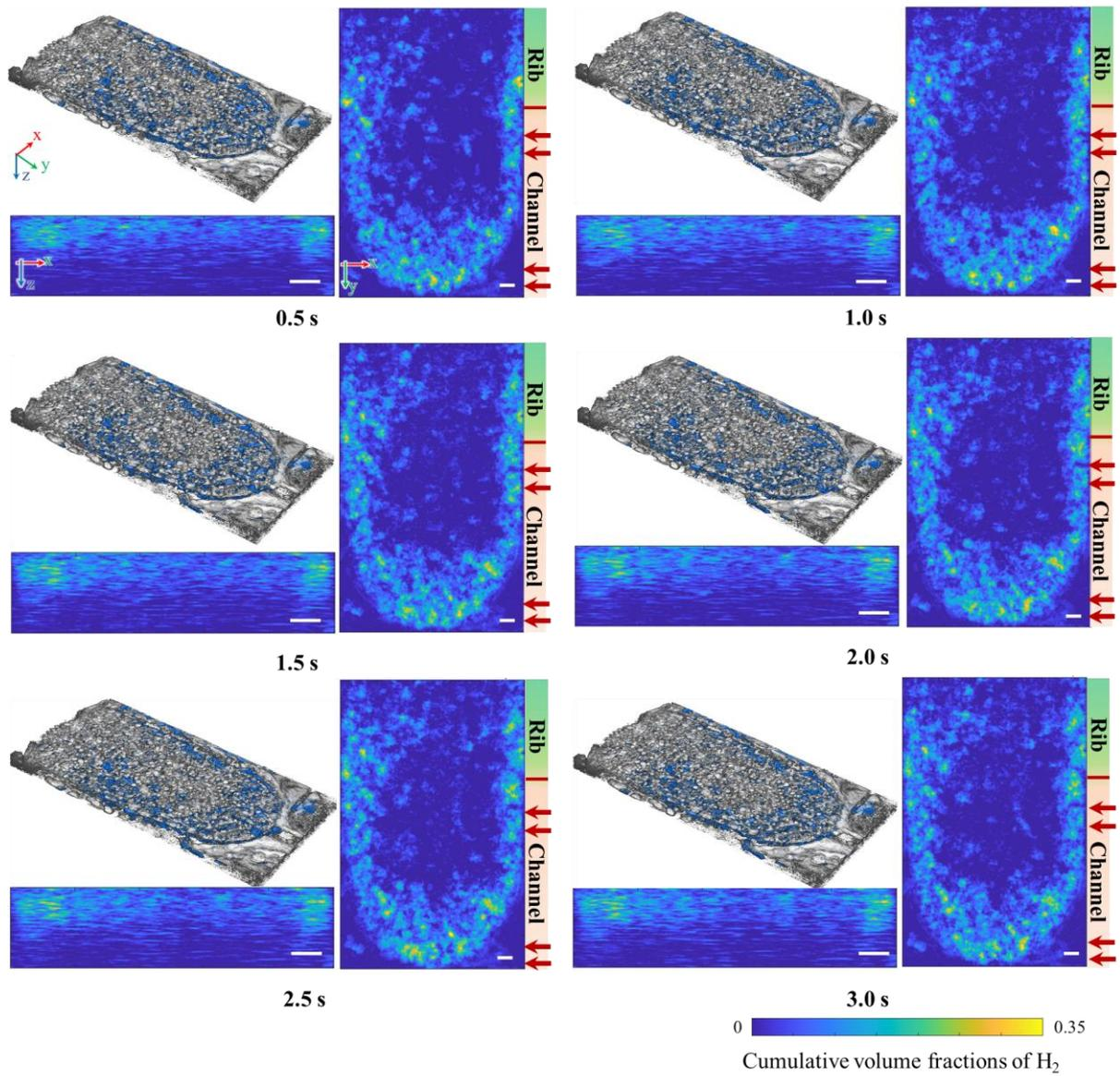
**Figure S10.** Time lapse images of the volume fraction of produced bubbles in the LNF at the current density of 80 mA/cm<sup>2</sup> and with the flow-by condition. Scale bar is 1 mm. The positions of the channel and the rib are given as well.
