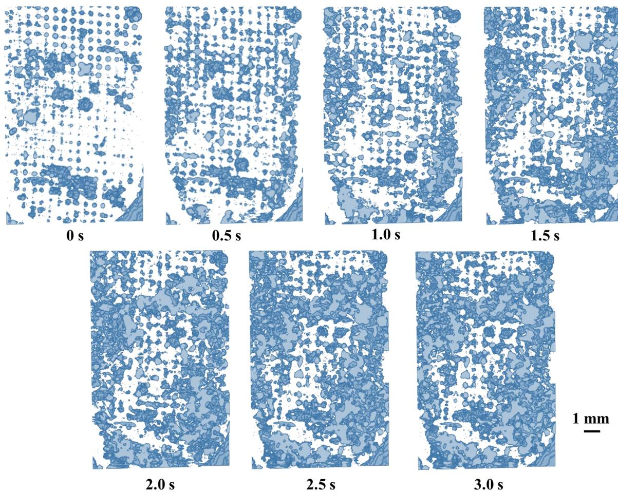
**Figure S5.** Time lapse images of the bubbles attached to the LNM at the current density of  $80 \text{ mA/cm}^2$  and without the flow-by condition.
