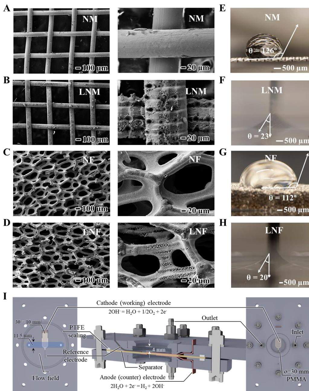
**Figure 1. The four investigated electrodes and the bespoke zero-gap flow-by AWE.**
