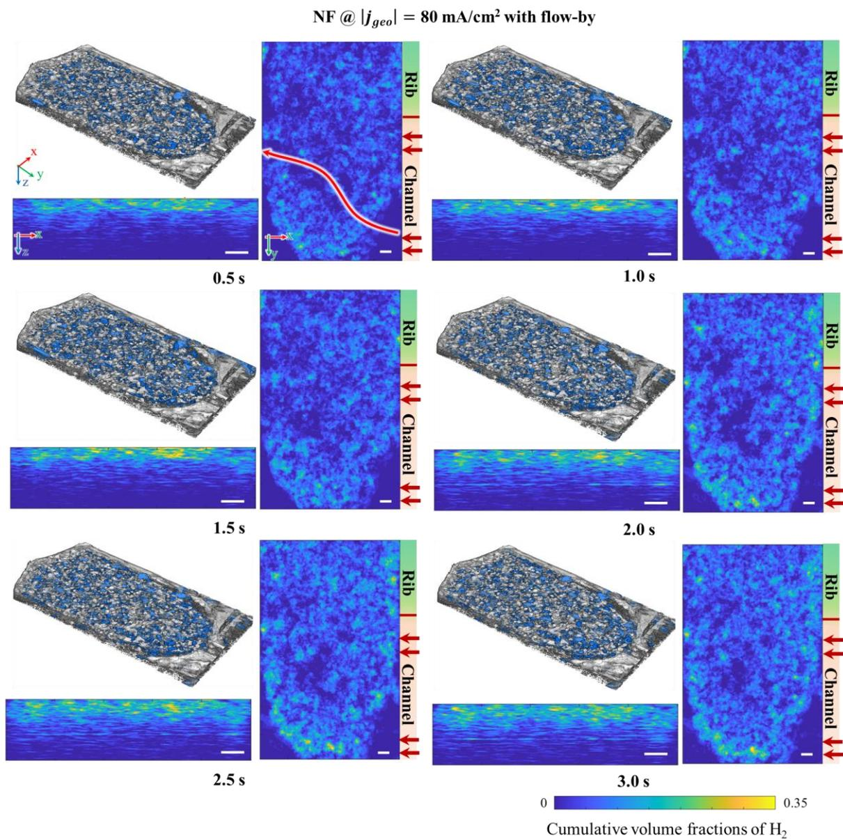
**Figure S8.** Time lapse images of the volume fraction of produced bubbles in the NF at the current density of 80 mA/cm<sup>2</sup> and with the flow-by condition. Scale bar is 1 mm. The positions of the channel and the rib are given as well. The red arrows show the flow-by direction. The low-resistance electrolyte pathway is more clearly observed as in the middle of the NF marked by the red arrow.
