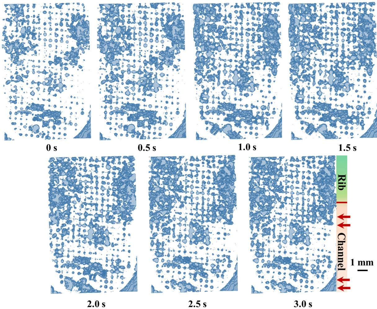
**Figure S6.** Time lapse images of the bubbles attached to the LNM at the current density of  $80 \text{ mA/cm}^2$  and with the flow-by condition. The positions of the channel and the rib are given as well. The red arrows show the flow-by direction.
