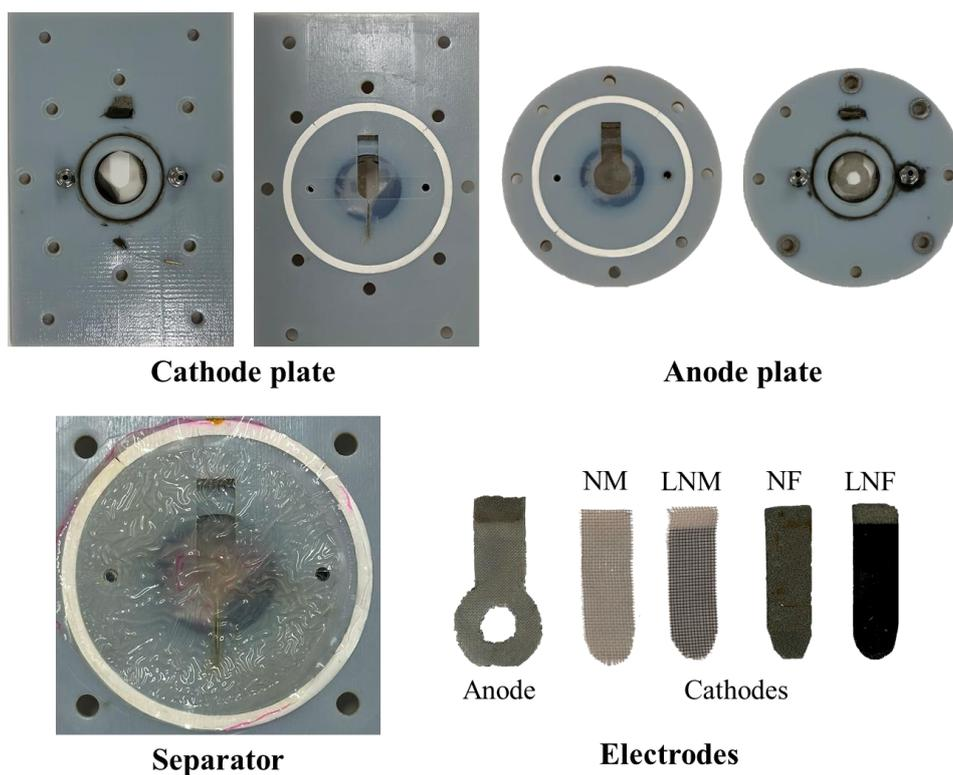
**Figure S1.** Images of the parts of the bespoke AWE, the ring shape counter electrode (anode) and the four investigated cathodic electrodes.
