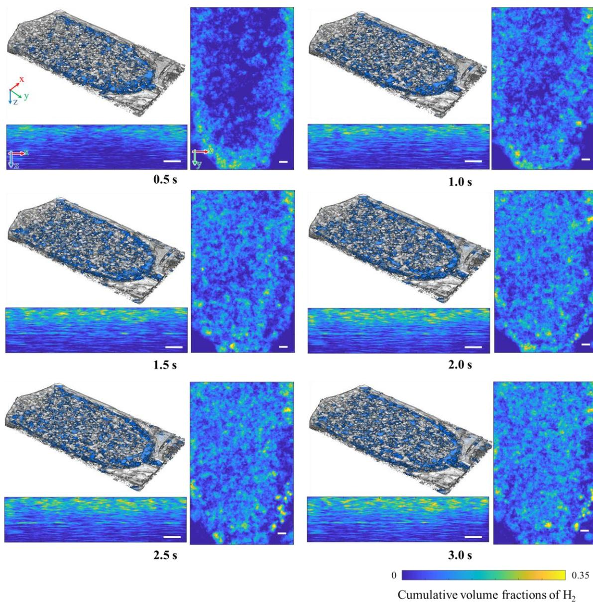
**Figure S7.** Time lapse images of the volume fraction of produced bubbles in the NF at the current density of  $80 \text{ mA/cm}^2$  and without the flow-by condition. Scale bar is 1 mm.
