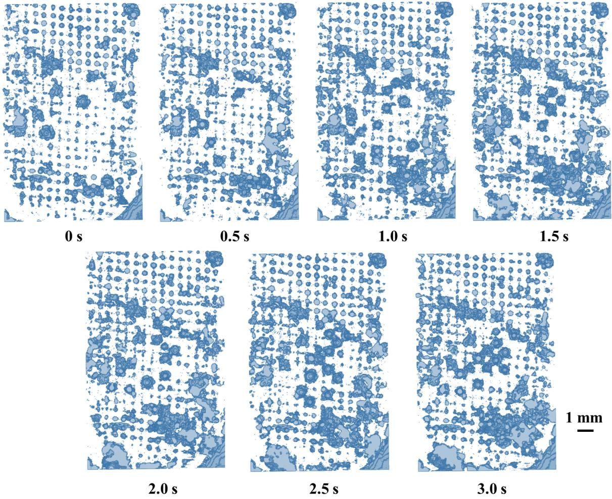
**Figure S4.** Time lapse images of the bubbles attached to the LNM at the current density of 40 mA/cm<sup>2</sup> and without the flow-by condition.
