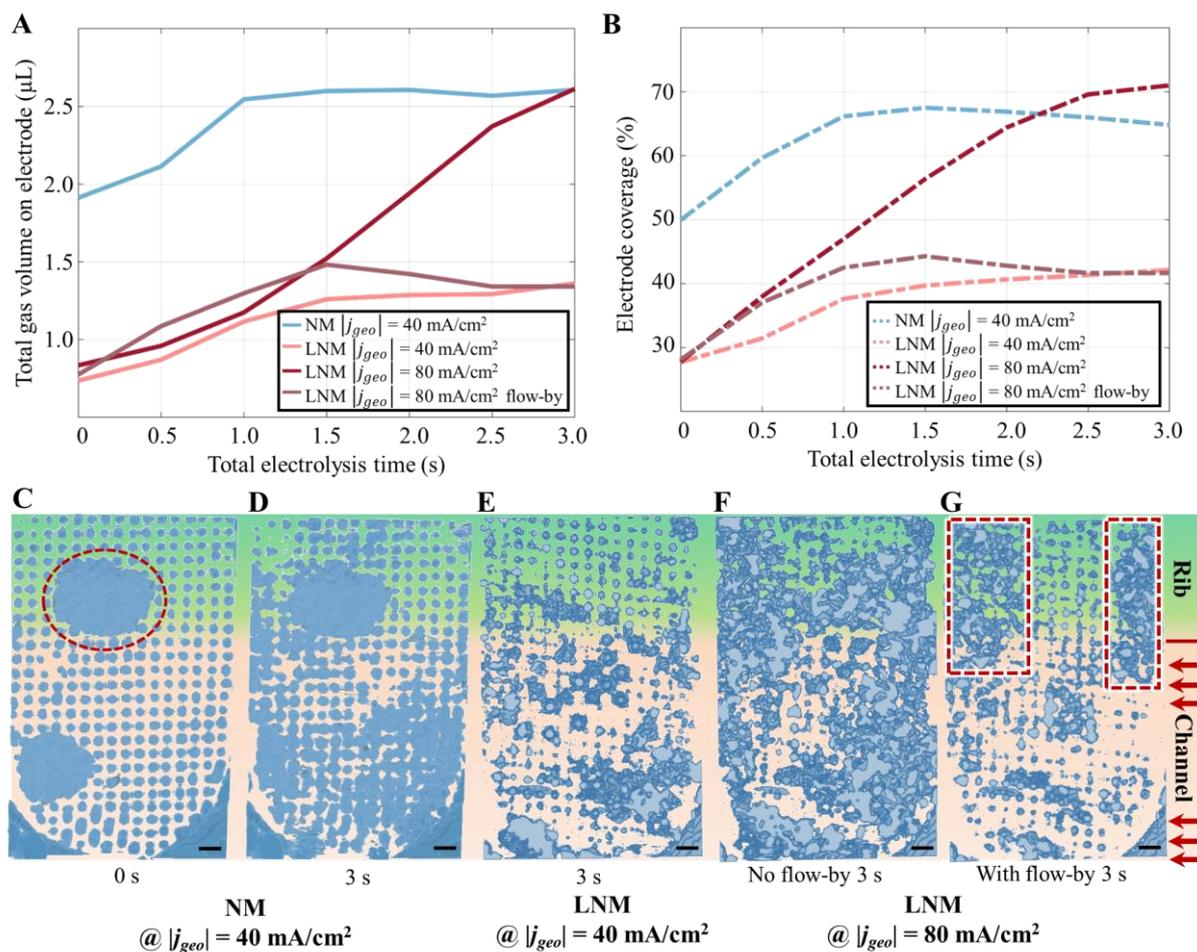
**Figure 5. Quantitative SAM visualizations of the gas bubbles on the NM and LNM.**
