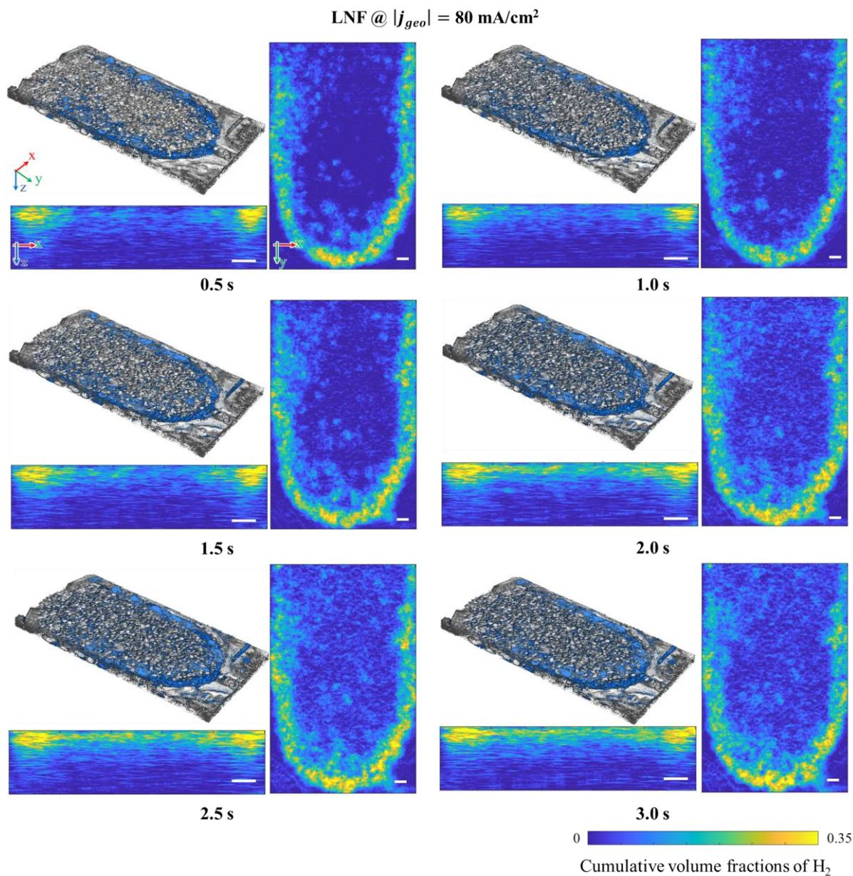
**Figure S9.** Time lapse images of the volume fraction of produced bubbles in the LNF at the current density of  $80 \text{ mA/cm}^2$  and without the flow-by condition. Scale bar is 1 mm.
