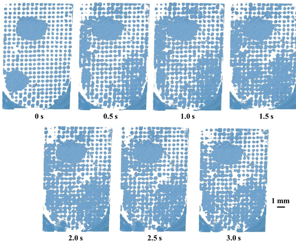
**Figure S3.** Time lapse images of the bubbles attached to the NM at the current density of  $40 \text{ mA/cm}^2$  and without the flow-by condition.
